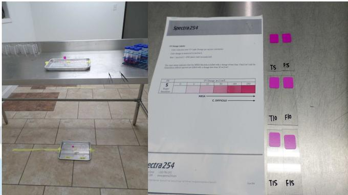
Left: Test carriers are held in place on tray for treatment. Photo shows carriers facing device at floor height and 3 feet. Carriers 5 feet from test device.
